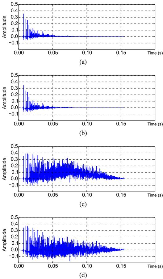
Figure 6: (a) Simulated room impulse responses. (a) Small reverberation ( $T_{60} = 70$  ms) without high-pass filtering. (b) Small reverberation ( $T_{60} = 70$  ms) with a sharp linear-phase high-pass filtering. (c) Strong reverberation ( $T_{60} = 400$  ms) without high-pass filtering. (d) Strong reverberation ( $T_{60} = 400$  ms) with a sharp linear-phase high-pass filtering.
