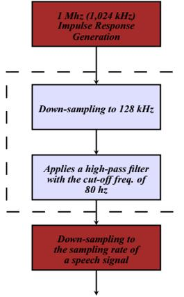
Figure 5: The procedure for calculating Room Impulse Responses (RIRs).
