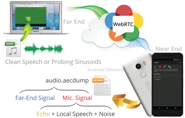
Fig. 2: AppRTC testbed for AEC data collection with Android devices.
