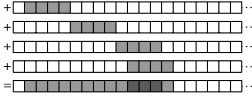
Figure 2. Example Loop Operation on 13 bytes. The first 12 bytes are copied using three non-overlapping 4-byte Block Operations. The remaining one byte is copied using a partially overlapping 4-byte Block Operation. Three bytes are accessed twice.
