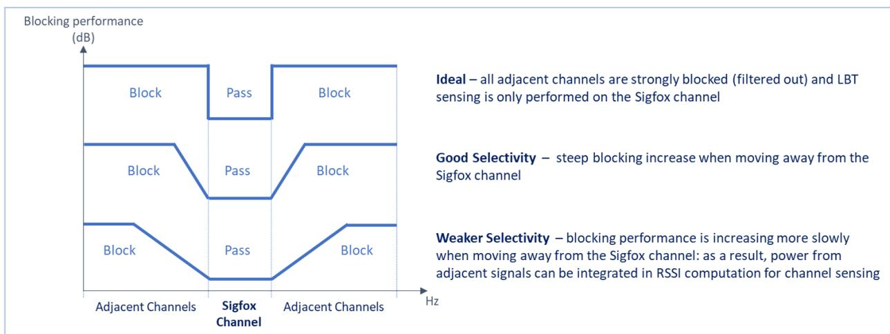
This **RSSI Selectivity or Blocking parameter** is fully dependent on the selected radio transceiver and device makers shall understand that the performance can widely vary from one provider to another.
