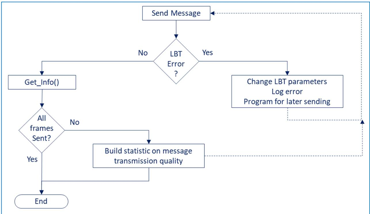
In the early phase of the deployment, during field tests/pilot, it is important to monitor the LBT mechanism both on device and backend side to build a learning database and tune the LBT mechanism to best suit the RF environment. This may require deploying a significant number of devices for a significant period as environmental parameters can widely change depending on location and overtime.
