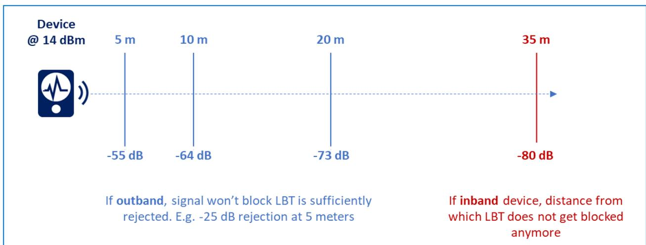
This chart is very theoretical: it assumes that other devices (transmitting in Sigfox or adjacent channels) can be localized. When deploying in dense urban area, a spectrum analyser could be used to assess the power of interferers in Sigfox channel as well as in adjacent channels.
