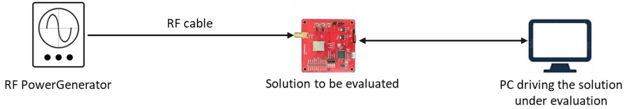
Use a RF power generator in continuous wave mode to generate strong interferers in adjacent channels and find the weakest power that blocks the device transmission starting from -40 dBm up to 0 or more.
