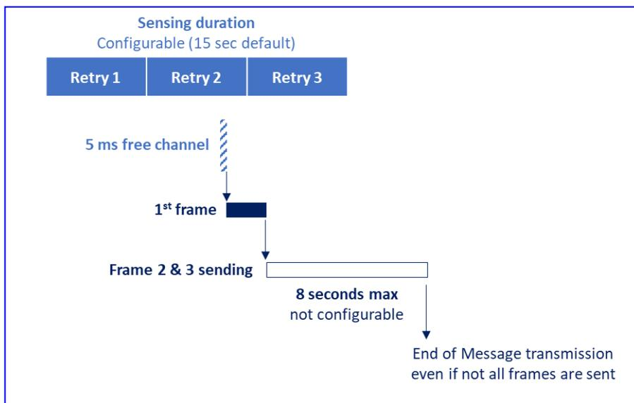
It is important to recall that LBT can block transmission possibly because of **outband** transmission (i.e. devices transmitting in adjacent channels). But it can also be blocked by **inband** transmission (i.e. devices transmitting in the Sigfox channel).
