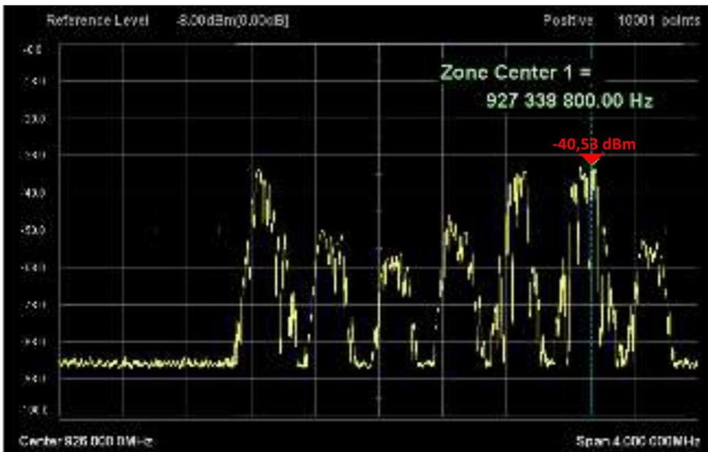
It is suspected that such RF noise could be generated by multiple Wi-Sun smart meters in very close proximity with the Sigfox device.
