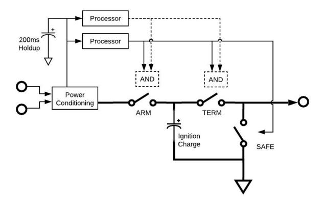
Normally a single processor controls a single termination output, however, as a factory option a logical AND can be added such that each termination output is voted upon by both processors.
