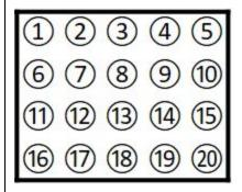
Face view of receptacle TE/DEUTSCH 732-8254-22. This connector is present on both the FTS-AIR and FTS-GND enclosures.
