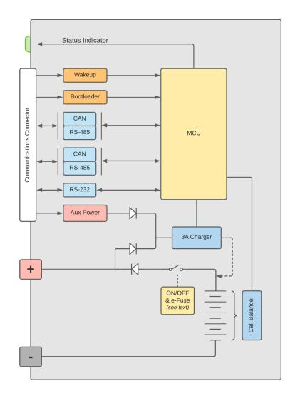
When the Lohner is at rest, the positive output terminal is electrically disconnected from the internal battery, described in this document as being in the "detached state". The MCU will operate in a low-power monitoring mode, checking for faults and monitoring the battery state-of-charge (SoC) and illuminating the externally visible fault indicator if a fault is detected. To conserve power at rest, communications interfaces are disabled.
