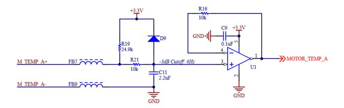
Both analog inputs are electrically equivalent to the above circuit. Alternate resistor configurations are available on request to achieve different gains.
