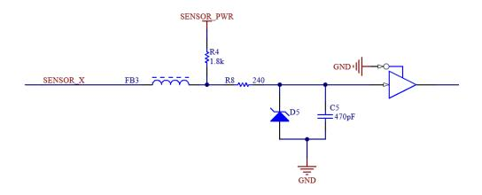
Each sensor input has a  $1.8 k\Omega$  pull-up for the case of open-collector output Hall sensors. The signal is also filtered through a  $240\Omega/470 pF$  (F<sub>C</sub> = 1.4 Mhz) RC low-pass filter. Then all 4 input sensor signals enter a logic buffer with <4.8ns delay.
