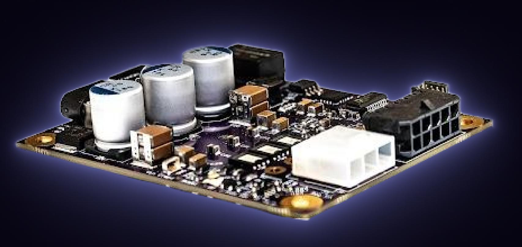
The Taurus AE (Actuator Edition) is a medium power, high efficiency BLDC motor controller that speaks in more than just pulses! This controller implements full FOC/SVPWM for highly efficient operation up to 2kW peak power and provides isolated CAN 2.0 and RS-485 communications, giving you more feedback and control of your propulsion system. The AE supports Hall or Quadrature sensor inputs for more accurate positioning.
