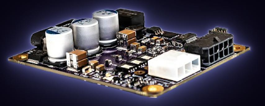
The Taurus AE (Actuator Edition) is a medium power, high efficiency BLDC motor controller that speaks in more than just pulses! This controller implements full FOC/SVPWM for highly efficient operation up to 2kW peak power and provides isolated CAN 2.0 and RS-485 communications, giving you more feedback and control of your propulsion system. The AE supports Hall or Quadrature sensor inputs for more accurate positioning.
