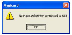
Check printer has power and the USB cable is connected
