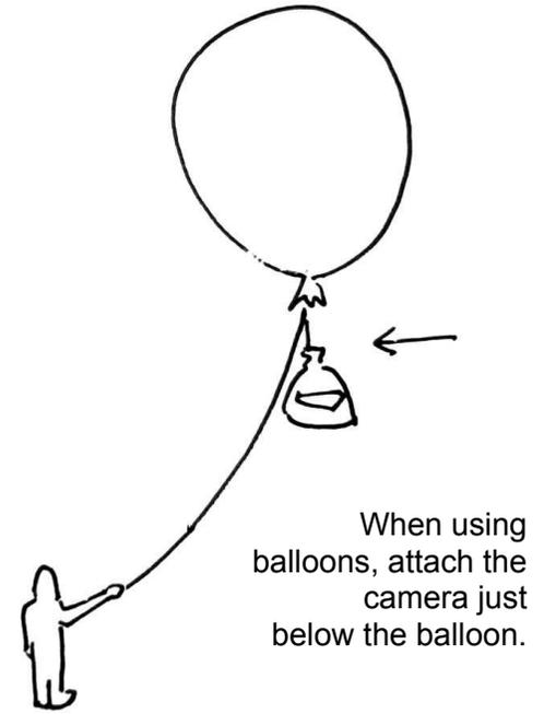
When using balloons, attach the camera just below the balloon.
