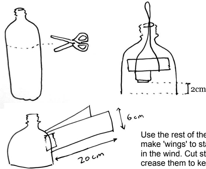
Cut a soda bottle in half and put the camera inside the top with the loop through the bottle neck.
