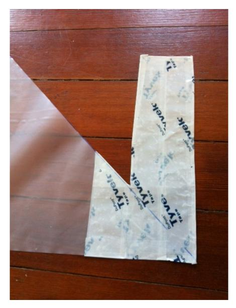
Tape both sides of the corner pockets with Tyvek tape, going slightly past the width of the pocket.
