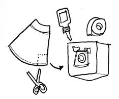
Cut a small square (~1cm square) of DVD-R close to the outer edge. Glue or tape it over the lens, keeping the track lines oriented vertically when viewed through the webcam -- parallel to the slit. Be careful not to get fingerprints on the DVD-R "diffraction grating" -- it acts as a prism to split the light into different wavelengths.
