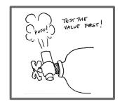
Test the valve, and lay the tank on the ground. Attach the regulator if one came with your tank (not pictured).
