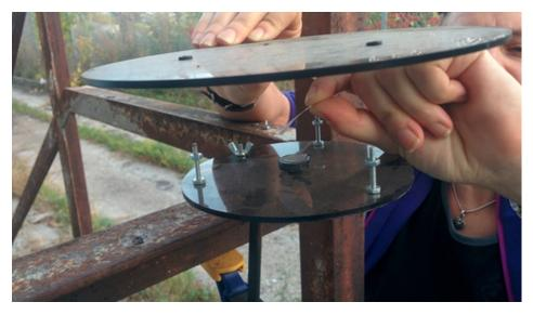
6) use the included bubble level to check if the housing is level. Reset the level of the housing using the thumb screw on the ball head.
