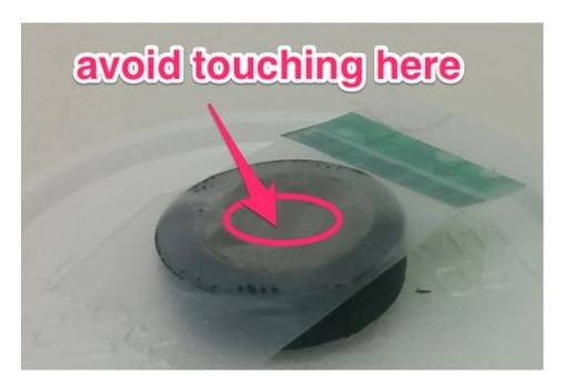
5) remove the sticky tab and immediately screw the housing's lid back on. The housing lid has a small groove on its underside that catches raindrops, make sure this groove is facing down.
