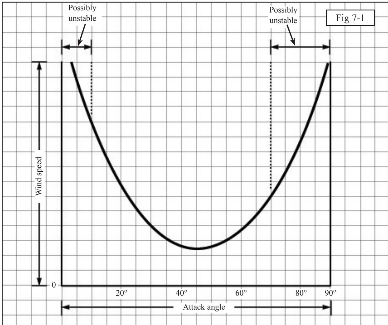
Attack angle vs minimum lift off wind speed and high wind instability (Guesstimated!).
