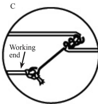
1" Paper clip made into 1/8"- 4 turn coil, 1/2" straight section then eyelet for string working end. Swing left to lock.
