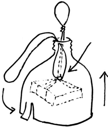
If you're using string, you can put the cap on over the string when the camera is snugly in place, trapping the string.
