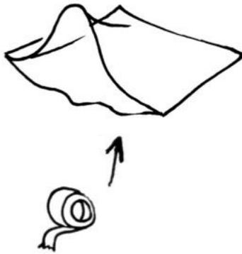
Where available, emergency mylar sleeping bags can be taped shut and, if carefully sealed, can stay filled for several days, unlike weather balloons. Two of these are enough to lift a typical camera.
