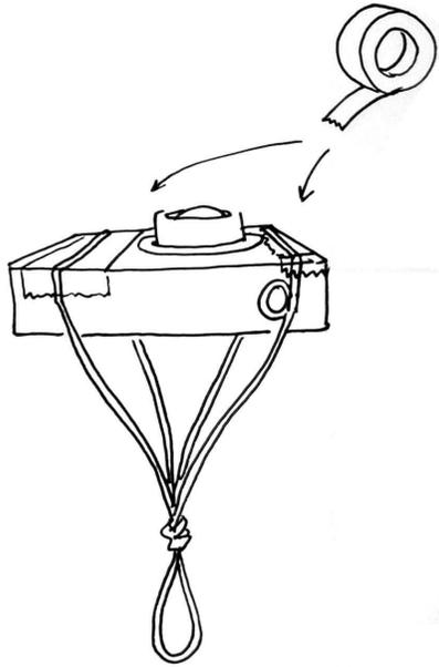
You can add a second loop or a rubber band and hook it on the bottom of the bottle to hold the camera firmly against the top.
