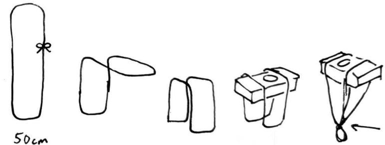
Press the tape down hard - it's the only thing keeping your camera from slipping out of the string at 500 meters high!
