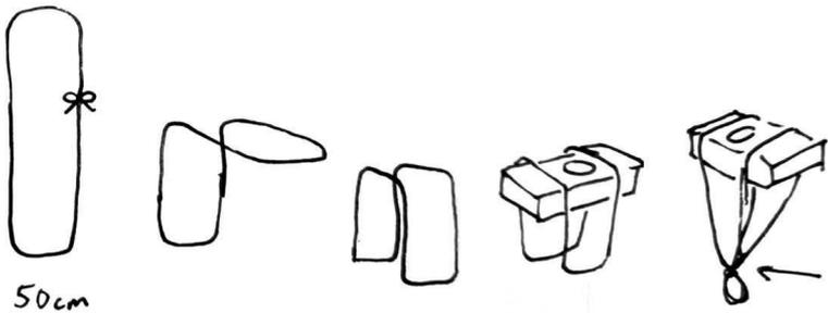
Press the tape down hard - it's the only thing keeping your camera from slipping out of the string at 500 meters high!
