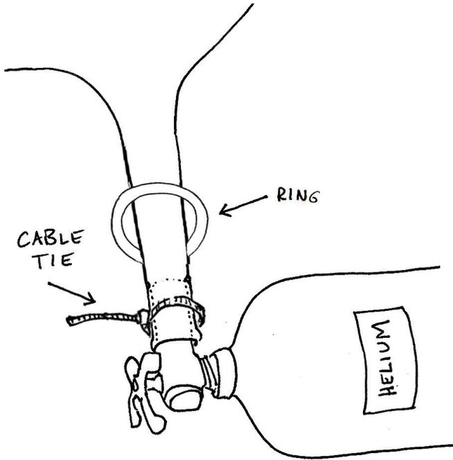
3. When you're done filling, push helium up out of the neck and close it with a removable zip tie (cable tie) or a very tight but untieable knot (shoelaces work well) just below the balloon.
