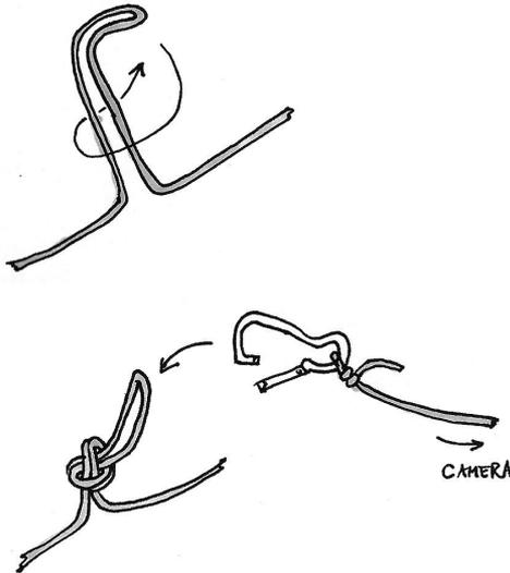
For kites, you don't need to make a tied loop; the tension of the kite pulling will hold a carabiner on if
