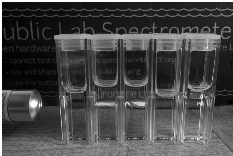
Several cuvettes in a row, demonstrating the way light should pass through them; photo by Jeff Warren (@warren)
