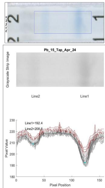
Figure 6: Computer Vision Strip Score Compared to Spiked Concentration
