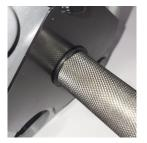
If dial lock is hard to move, unscrew bolt slightly. Dial lock should move but not be loose.
