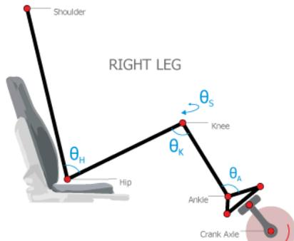
**Figure 2:** Schematic illustration of a participant's right leg, with joint angles defined as: hip ( $\Theta_H$ ); knee ( $\Theta_k$ ); knee splay ( $\Theta_S$ ); and ankle ( $\Theta_A$ ). Retroreflective markers are marked by red circles.
