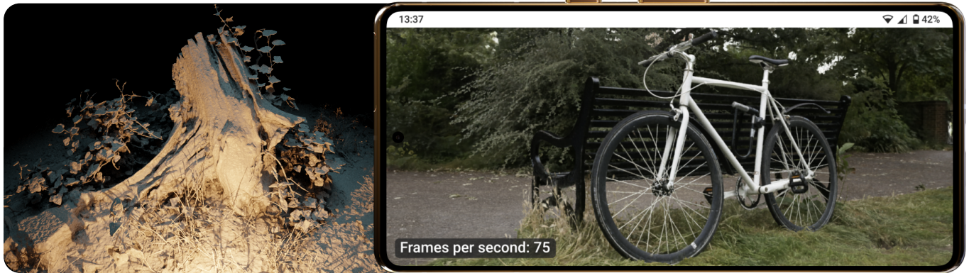
Fig. 1. Our method reconstructs triangle meshes from multi-view images and is able to capture fine geometric detail such as leaves, branches and grass (left). At the same time our meshes are compact enough for real-time view synthesis on a Google Pixel 8 Pro (right).
