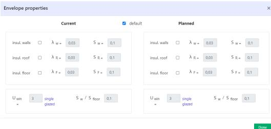
The "envelope &wins" button lets the user directly choose the thickness and the thermal conductivity of the wall (and roof) insulation and to explicitly provide values to the window transmittance and to the ratio between windowed and floor surfaces.
