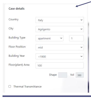
By checking the "Thermal Transmittance" check box, it is possible to modify also two important properties: the height and the ratio between dispersing area and volume. The value of this last parameter is paramount for a correct calculation of the thermal losses. The default value is to be verified accurately since it depends on building type (e.g., n. of floors), age and location (architectural custom). Furthermore, you can define transmittance values different from those uploaded in the
