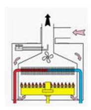
**Sealed Chamber**. The combustion chamber is sealed and it has no contact with the surrounding environment. Air for the combustion is taken outside by using a ventilation system and exhaust gases are expelled outside. This boiler can be installed in an internal environment.
