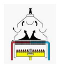
**Open Chamber**. This boiler takes the air necessary for the combustion from the surrounding environment, therefore the combustion chamber is connected with the surrounding environment. The exhaust pipe is usually vertical and transports the exhaust gases outside. Usually these boilers should be installed outside in order to avoid the risk of forming carbon monoxide in the internal environment.
