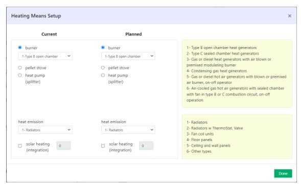
The "heating" button opens the form dedicated to the selection of the heating generators, the heat emitters (radiators, fan coils, etc.) and of the potential solar thermal integration.
