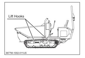
1. Attach hoisting slings to 4 lift hooks located on the corners of the machine. Hoist the center of the slings.
