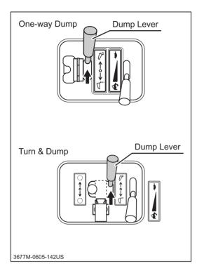
One-way Dump Lock Plate Turn & Dump Lock Plate Lock Plate Lock Plate Dump Lever Dump Lever Move dump lever gradually toward [<sup>1</sup>/<sub>1</sub> (up)] to raise bucket.
