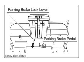
With parking brake pedal depressed, pull out parking brake lock lever to lock parking brake.
