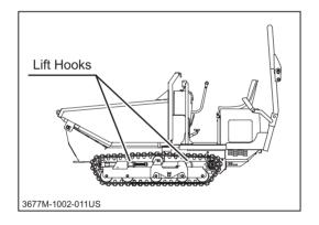
5. Tie the machine at lift hooks with rope or tiedown belts and secure it onto the loading deck of the transporter securely.
