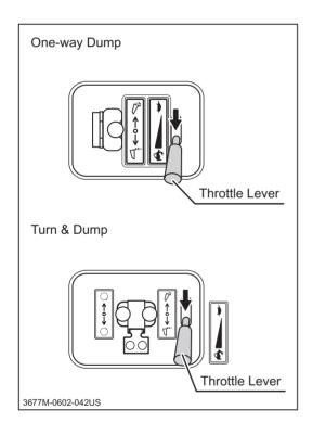
Push throttle lever to [ (fast)] position to increase engine speed.
