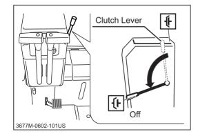
6. Move clutch lever to [{+(off)] position.
