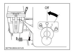
3. Turn main switch to [ () (off)] position and remove key from main switch.
