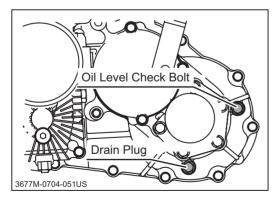
3. Remove oil level check bolt. Check that oil level is at the check bolt hole.
