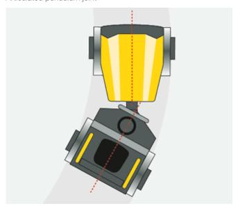
**Uniform compaction, optimal driving stability:** The three-point articulated pendulum joint ensures a uniform weight distribution on the front and rear drum at all times. This also improves the maneuverability and provides for maximum tipping safety and stability when turning curves.
