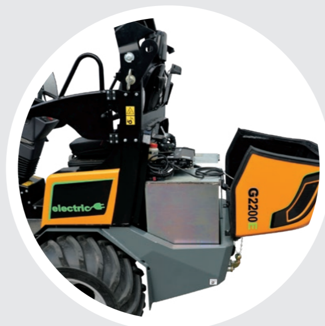
Energy recuperation: automatic charging of the battery, e. g. during braking processes
