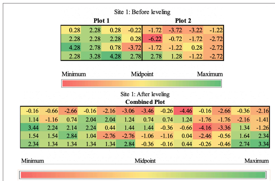
Figure 4. Comparison of mean elevation (cm) in Site 1 before and after land laser leveling.
