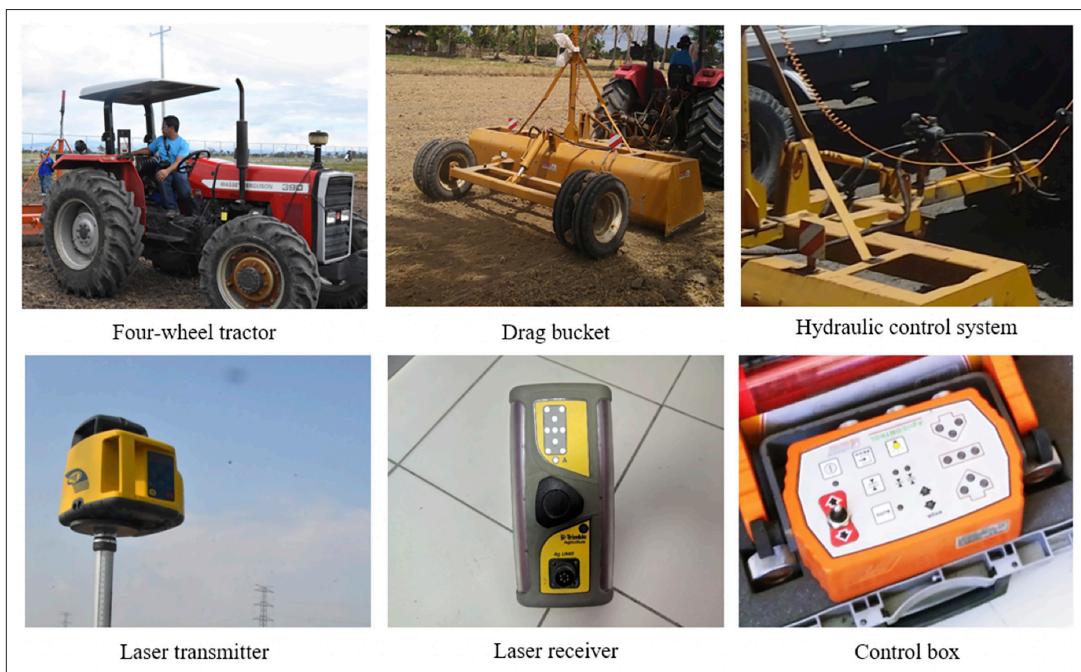
Figure 3. Components of a Laser land leveling system.
