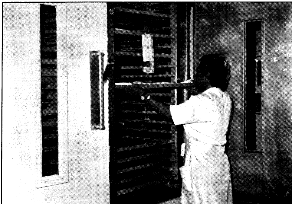
Figure 11. Drying of Extracted Pectin at 60°C in Fabricated Drying Oven.
