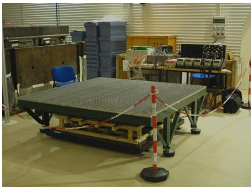
Figure 2. Muon monitor in assembled state alongside with shielding.
