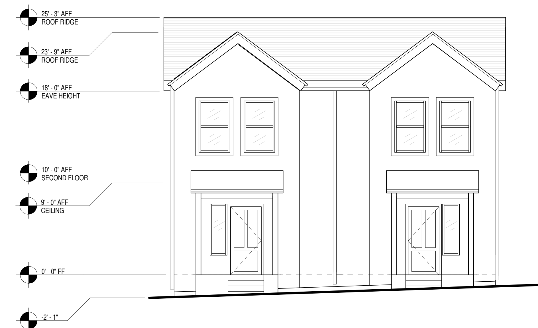
A3 EAST ELEVATION - BUILDING A SCALE: 3/16" = 1'-0"
