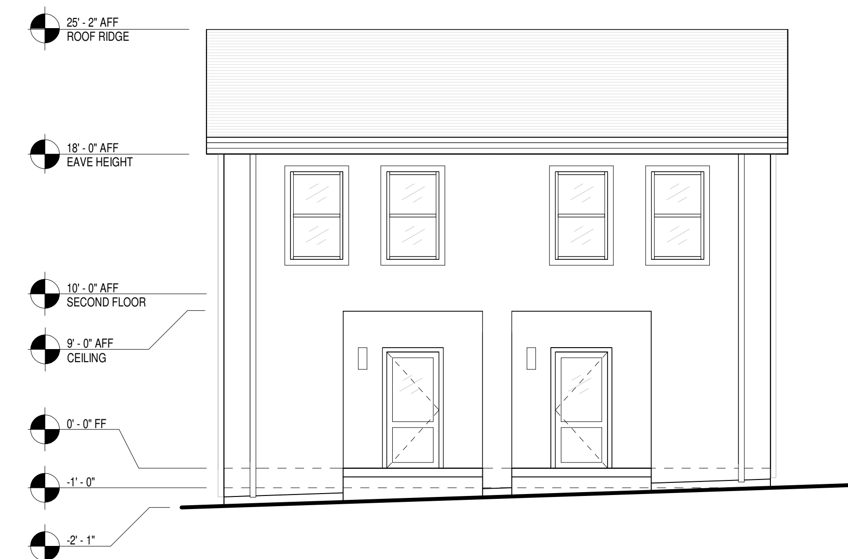
C3 WEST ELEVATION - BUILDING A SCALE: 3/16" = 1'-0"
