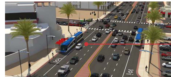
Side-Running BRT Station
