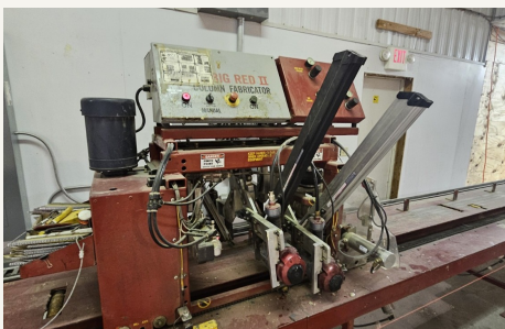
COLUMN FABRICATOR / LAMINATOR
