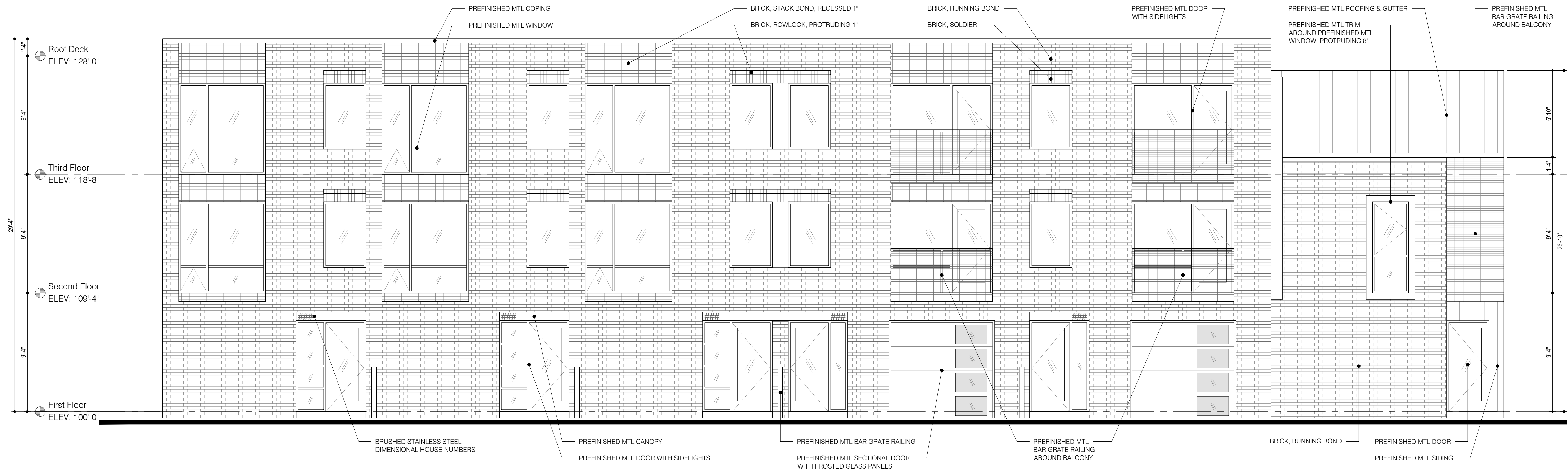
1 West Elevation - Beaubien St. A401 Scale: 1/4" = 1'-0"
