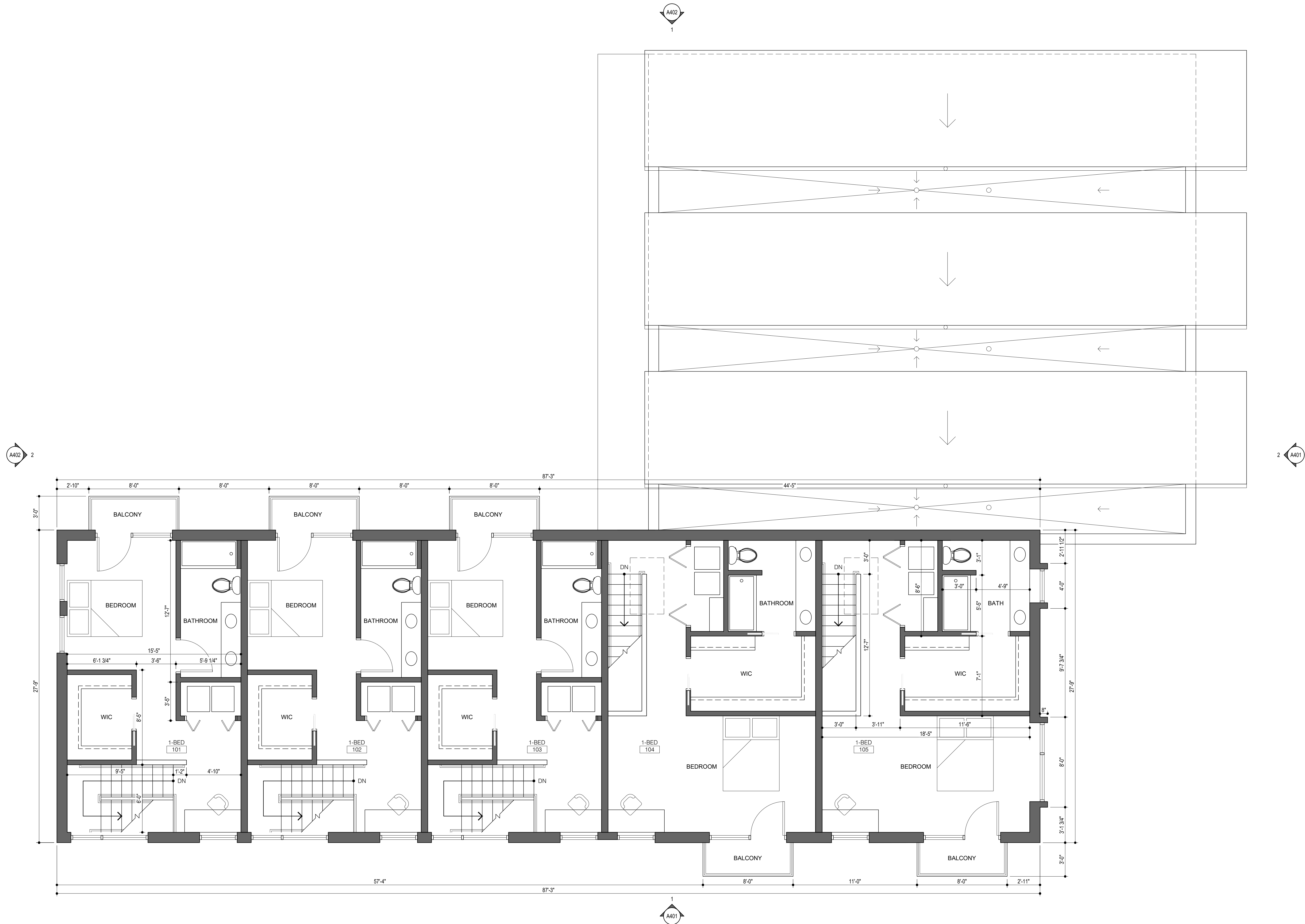
1 A203 Third Floor Plan Scale: 1/4" = 1'-0"
