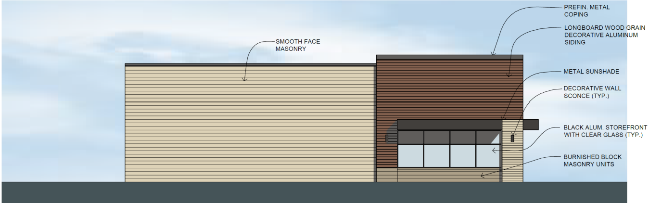
West Elevation Scale: 3/32"=1'-0"
