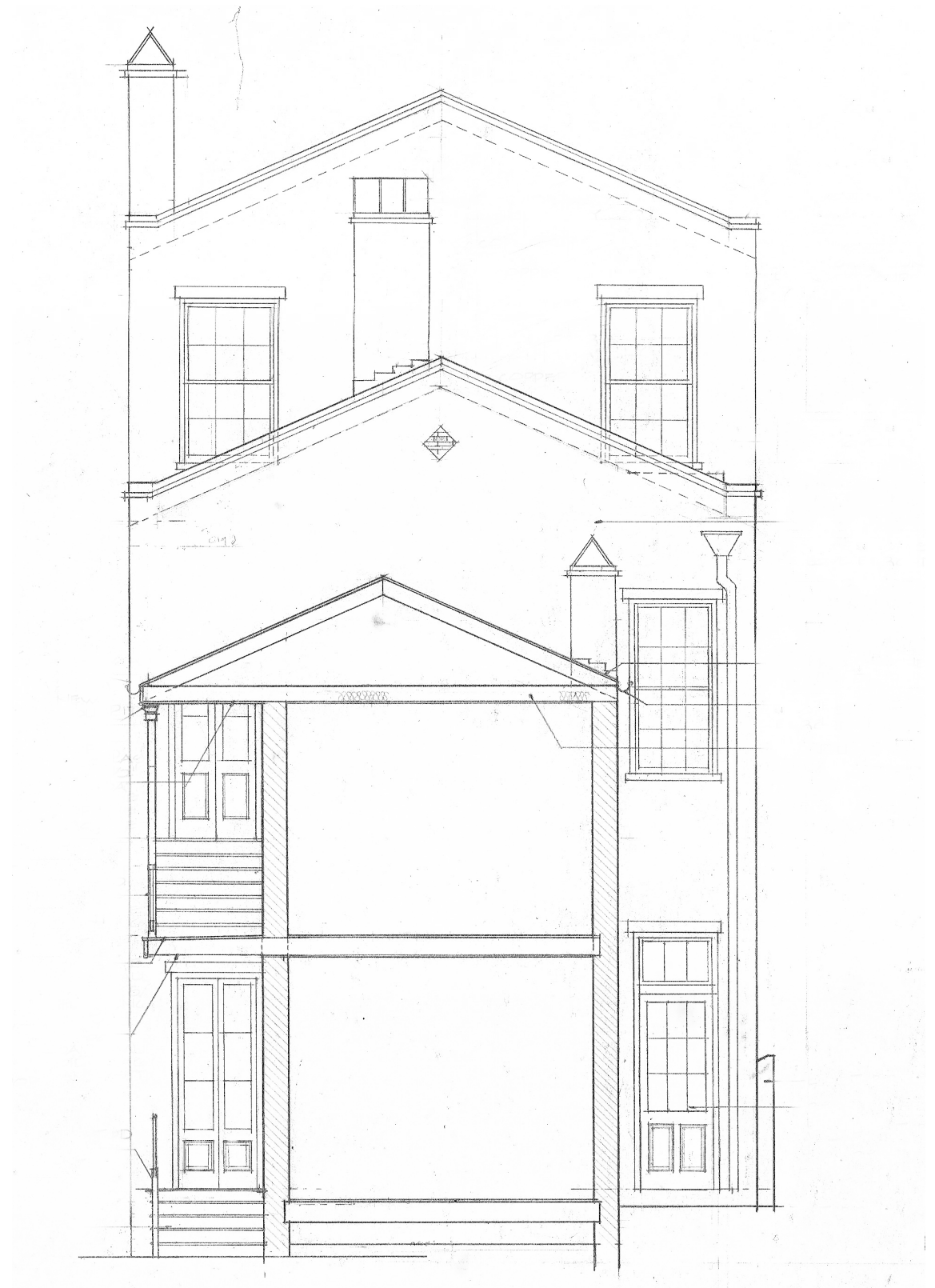
rear elevation / section
