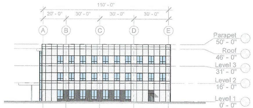
④ NORTH EXTERIOR ELEVATION (S.D.) 1/32" = 1'-0"
