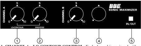
**1. CHANNEL A: LO CONTOUR CONTROL:** Each channel is equipped with a LO CONTOUR control. This control is a low frequency adjustment for the BBE 262. It provides a boost of 10dBu when turned to its maximum position (clockwise) at 50Hz. When turned to its minimum position, (counter-clockwise), the low frequency is flat.
