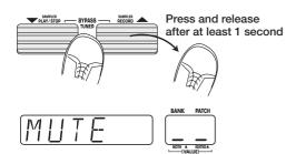
The indication "--" on the BANK/PATCH indicator shows that the tuner is in the input standby condition.
