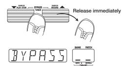
While the BFX-708 is in the bypass condition, the amp simulator is also off and the expression pedal works as a volume pedal.
