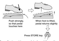
The adjustment is completed, and the unit returns to the play mode.
