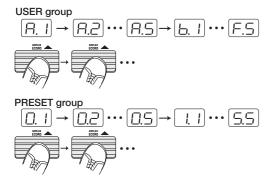
2 To directly switch the bank, use the TYPE (BANK) ▼/▲ keys. This allows you to move to the next lower or next higher bank.
