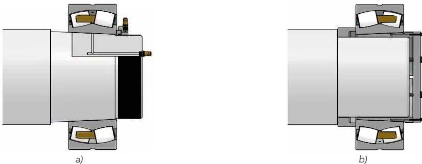
Hydraulic methods for mounting tapered bore bearings: a) hydraulic nut b) special sleeve
