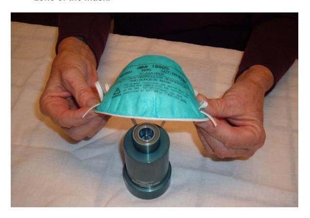
4. Place upper handle/grommet holder on mask. Note: internal magnets will center the grommet.
