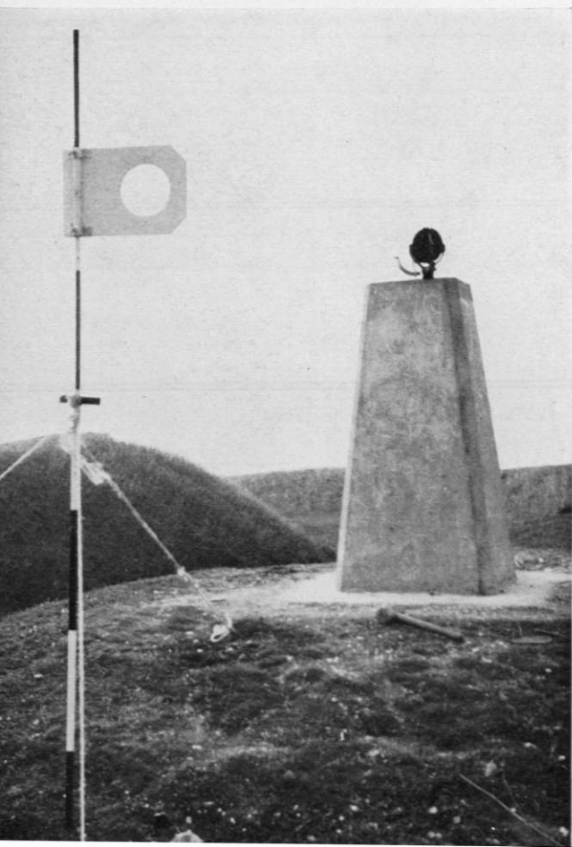
Heliotrope, with duplex mirror in use, and semaphore board
