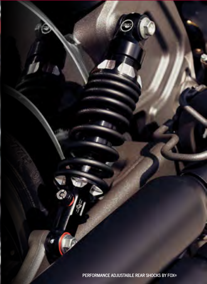
ADJUSTABLE PIGGYBACK REAR SHOCKS
