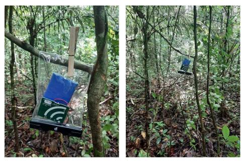
**Figure A2.** The AudioMoth device, an open acoustic, lightweight, and affordable autonomous recording unit used to monitor the soundscape in Puerto Rico during 2021. The device hardware, which included a lithium-ion rechargeable battery (blue packet in the photo), was placed in a protective waterproof plastic case with a silica packet and then deployed in a tree/vine/shrub at a 1.5 m height.
