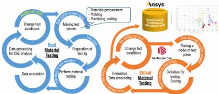
Fig. 1 - Comparison of virtual and numerical material testing with a focus on cost.
