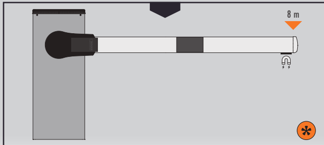
boom with internal joint and magnet
