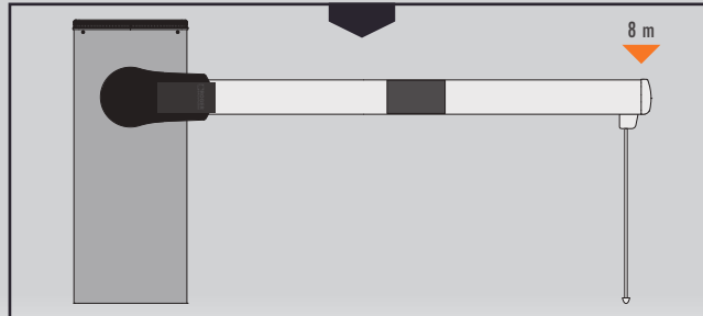
boom with internal joint and rest
