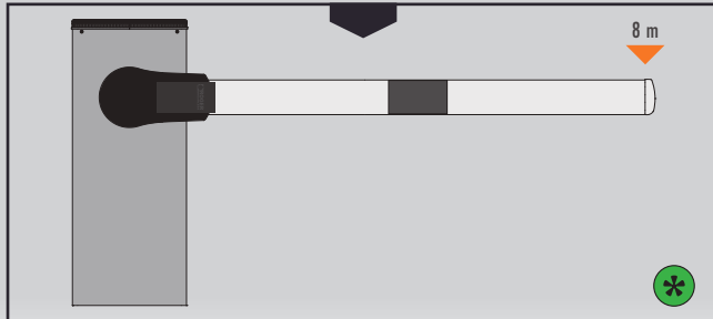
boom with internal joint
