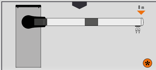
boom with internal joint and magnet
