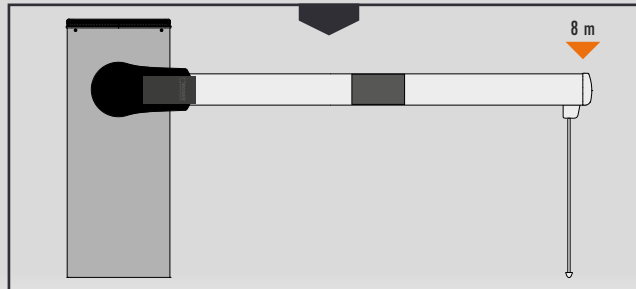
boom with internal joint and rest
