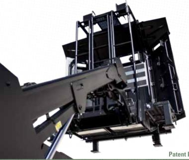
When the Armored Deployment Platform is mounted on the vehicle, the operator can raise it to 11 feet (to the bottom of the platform) so that entry can be made on the first, second, and third floors. The platform height is also ideal for airplane assault incidents. In a vehicle take down, the platform can be slanted downward for crowd control and rescues.
