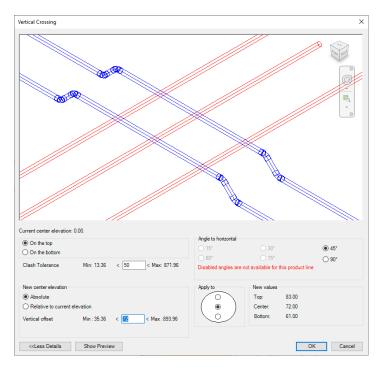
Note that the pipes/ducts/cable trays that are going to be adjusted need to be parallel with each other and parallel with the level. Sloped systems are currently not supported. Also the references have to be in parallel with the level as well.
