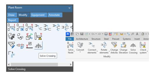
2. Select the duct/pipe/cable tray that has to be adjusted and press Finish.
