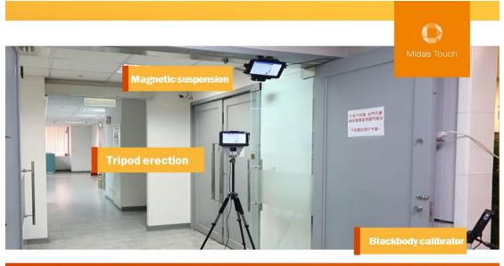
MTA-3078T consists of a rugged touch panel, a compact FLIR thermal imaging camera, and a dynamic temperature calibrator. With MTA-3078T, you no longer need to stare at the screen to observe the inspected persons.
